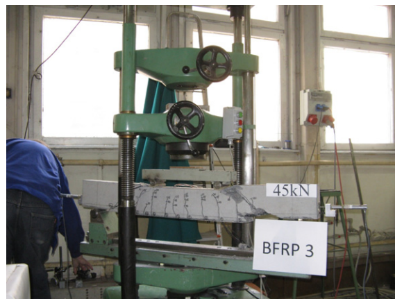
Fig. 4. The beam with flexural BFRP reinforcement with load capacity 45 kN [14]
