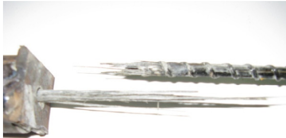
Fig. 2. Basalt bar (8 mm in diameter) after rupture in tension test [14]
